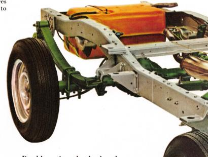
**Double-acting shock absorbers**—both front and rear—further dampen road shock and increase handling ease.
