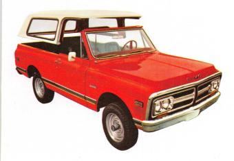
Removable fiberglass hard top is an extra-cost option that turns Jimmy into an all-weather station wagon. Features full side windows, rear upper lift gate and black or white textured paint finish. A folding soft top is also available.
